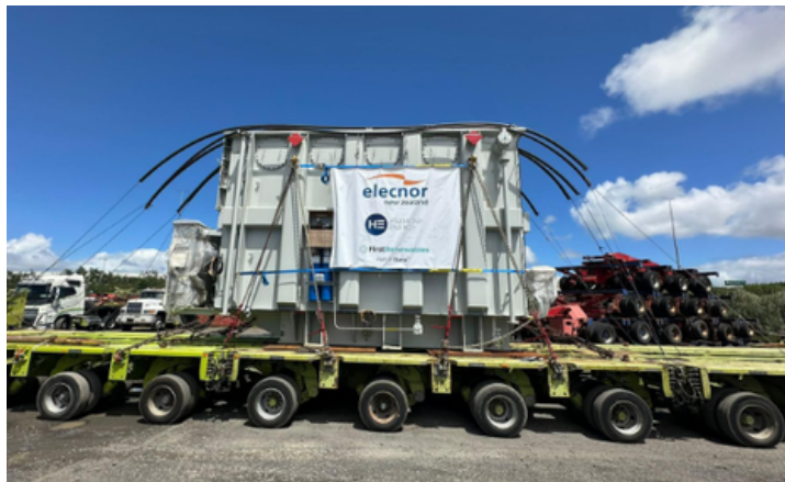
Oversize transformer arriving on site on a 17-axle, 56 metre long truck
